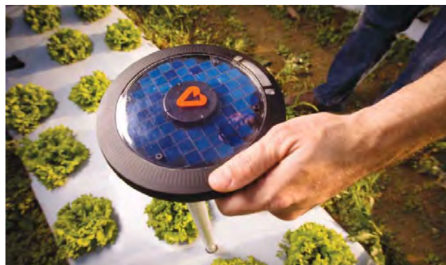
Figure 28 Arable's device that combines weather and plant measurements in real-time 81
